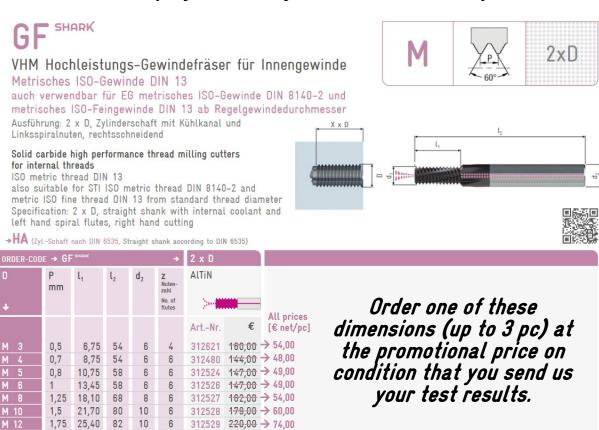
The high-performance thread milling cutter type SHARK represents a central further development at JBO. It was designed as a **standard tool for universal use in general mechanical engineering** for machining steel materials. Further areas of application are the machining of cast materials, titanium alloys and non-ferrous metals.
